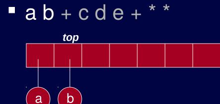
If symbol is an operand, put it in a one node tree and push it on a stack.
