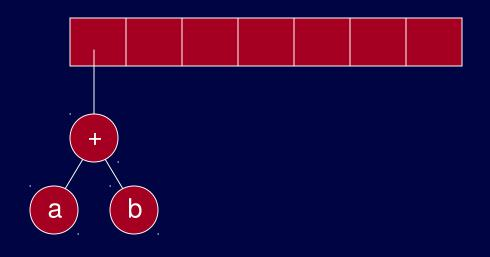
If symbol is an operator, pop two trees from the stack, form a new tree with operator as the root and  $T_1$  and  $T_2$  as left and right subtrees and push this tree on the stack.
