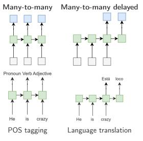
For recurrent nets, loss is between *series* of output and target vectors. That is  $\mathcal{L}(\{\mathbf{y}^{(1)}, \dots, \mathbf{y}^{(T)}\}, \{\mathbf{t}^{(1)}, \dots, \mathbf{t}^{(T)}\})$ .
