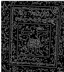
Figure: Neither the high threshold alone ( left ) nor the low threshold alone ( middle ) is sufficient for good edge detection. Right: Order of visiting pixels during hysteresis thresholding. Darker corresponds to pixels visited earlier. Bottom row is for the noisy image. Author: N. Khan (2021)
