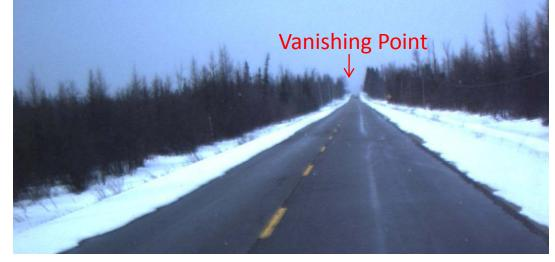
Why do parallel lines meet in a projected image? (Hint: use the projection equations x=fX/Z and y=fY/Z)
