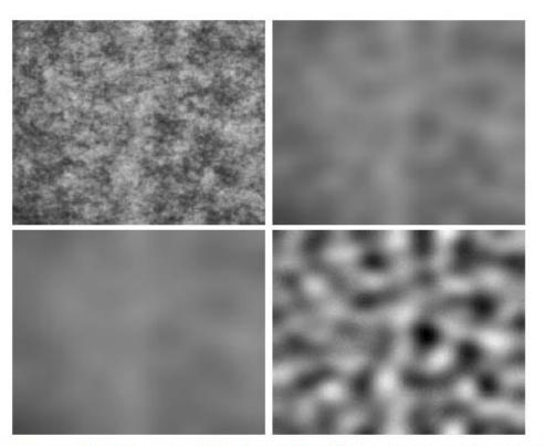
(a) Top left: Fabric,  $257 \times 257$  pixels. (b) Top right: After lowpass filtering with a Gaussian with  $\sigma = 10$ . (c) Bottom left: Lowpass filtering with  $\sigma = 15$ . (d) Bottom right: Subtracting (b) and (c) gives a bandpass filter that visualises cloudiness on a certain scale. The greyscale range has been affinely rescaled from [-13, 13] to [0, 255]. Author: J. Weickert (2002).
