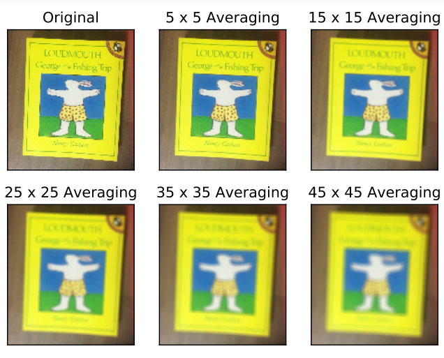
Figure: Effect of convolving with averaging masks of increasing size. Author: N. Khan (2018)
