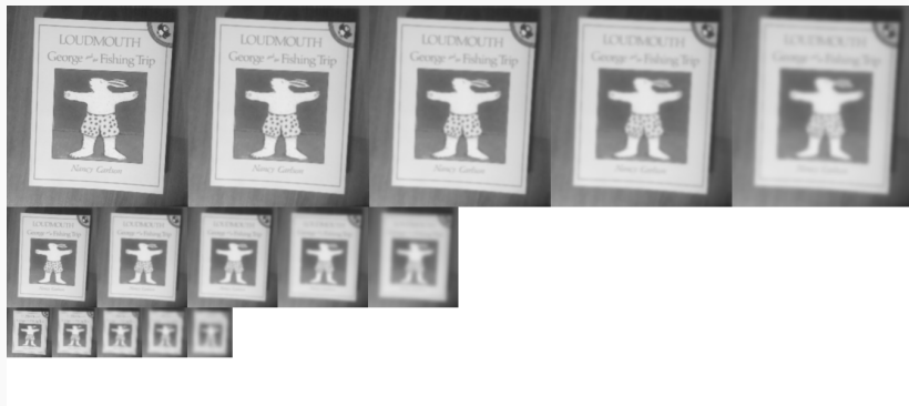
Figure: A Gaussian pyramid with 3 levels and 5 smoothing scales. Top to bottom: Subsampling in both dimensions by factor 2^i for i = 0, \dots, 2 . Left to right: Gaussian blurring with \sigma = \sqrt{2^j} \sigma_0 for j = 0, \dots, 4 and \sigma_0 = \sqrt{2} . Author: N. Khan (2018)
