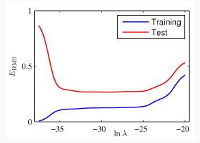
Graph of root-mean-square (RMS) error of fitting the M = 9 polynomial as  $\lambda$  is increased.
