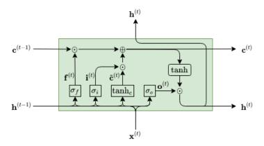
LSTM Cell: Operations at the hidden layer in detail.
