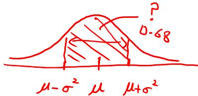
$$z = \frac{x - \mu}{\sigma} \leftarrow \begin{array}{l} z\text{-transformation} \\ \text{standardization} \end{array}$$
