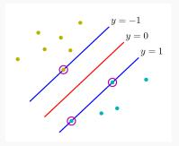
**Figure:** The margin is defined as the perpendicular distance between the decision boundary and the closest of the data points, as shown on the left figure. Maximizing the margin leads to a particular choice of decision boundary, as shown on the right. The location of this boundary is determined by a *subset of the data points*, known as *support vectors*, which are indicated by the circles.
