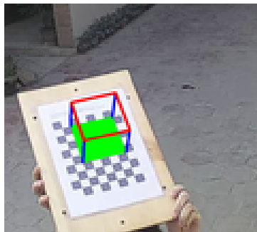
Figure: A 3D cube augmented onto the plane of the calibration checkerboard in two different orientations. Author: N. Khan (2018)
