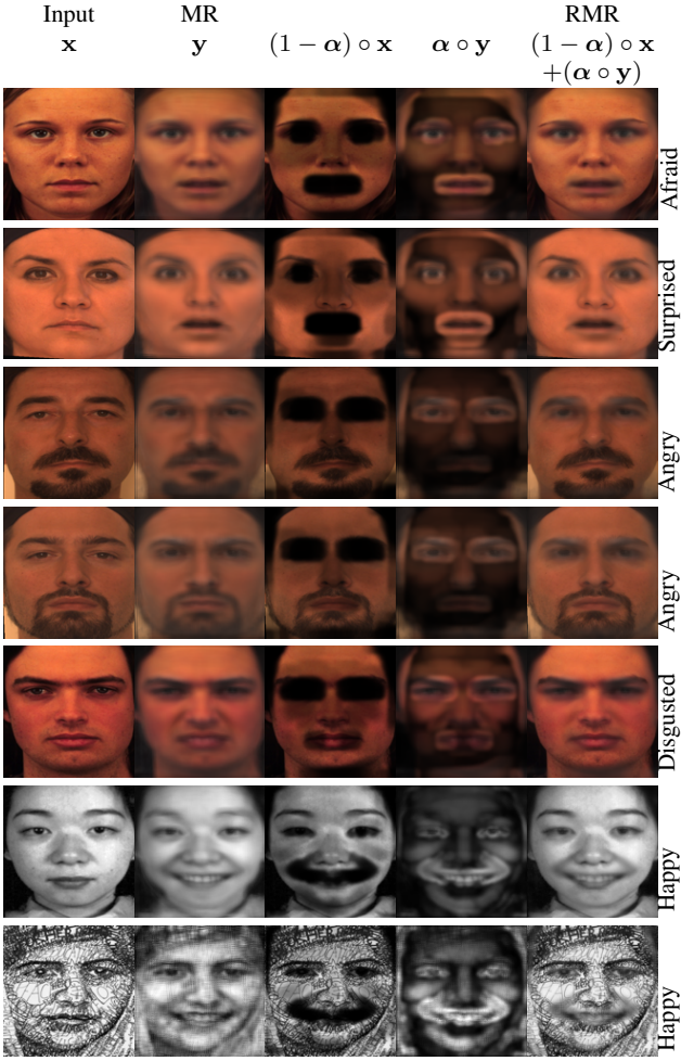
Fig. 16 Visualization of the blur refinement algorithm as explained in Section 6. Image details from input x and expression details from MR output y are used to yield a refined expression image. The refined results show better recovery of facial hair, illumination effects and subtle facial features. An overall improvement in identity preservation can also be observed. The input image in the last row is made by combining different letter strokes. In the refined result, many of the letter strokes are also recovered (zoom in for better view).
