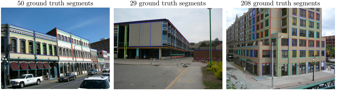
FIGURE 4: Manhattan bias and incompleteness of ground truth marked in YorkUrbanDB [15]. Many valid segments with strong underlying image gradients are not marked since they do not belong to significant building boundaries. For example, vehicles, pavements, small light poles, and small window boundaries are ignored.
