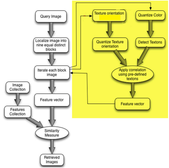
Fig. 3: Flowchart of the the propose algorithm. The area is yellow represents the iterative process carried out on each block.
