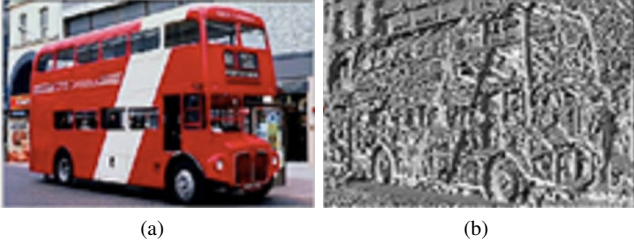
Fig. 2: (a) An input image, (b) Texture orientations of (a).
